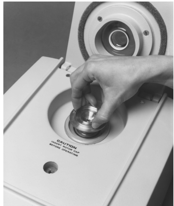
Figure 5-2. Lifting Out the Stator. Keep the stator level to prevent binding.
