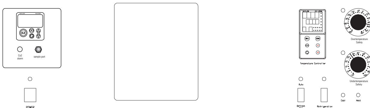
Figure 2-1. Environmental Chamber Control Panel (shown with optional CO 2 control)
